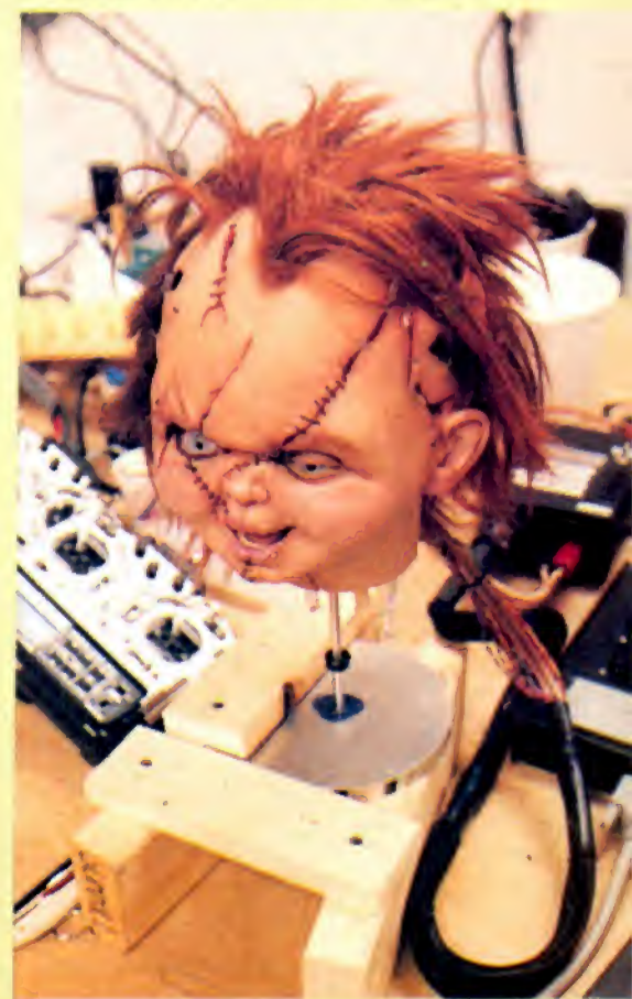
Chucky’s cable-controlled animatronic head, requiring eight operators for prerecorded dialogue.
